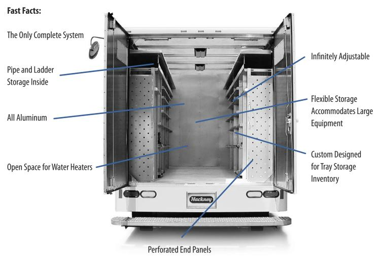
Shelves shown installed in the complete Hackney AC1000 body. Now available as a complete system or for retrofit
